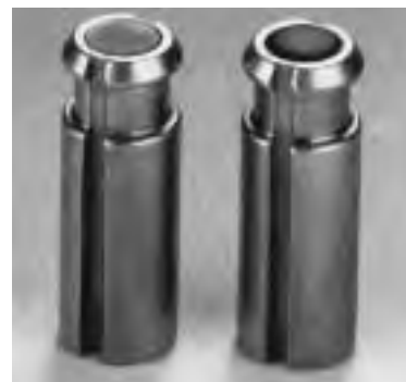
Solenoid valve plunger travel stroke is typically 0.020 to 0.050 in., depending on orifice size. Choosing the wrong seal material could literally shut off the valve flow. Notice the swelling in the seal at right.
